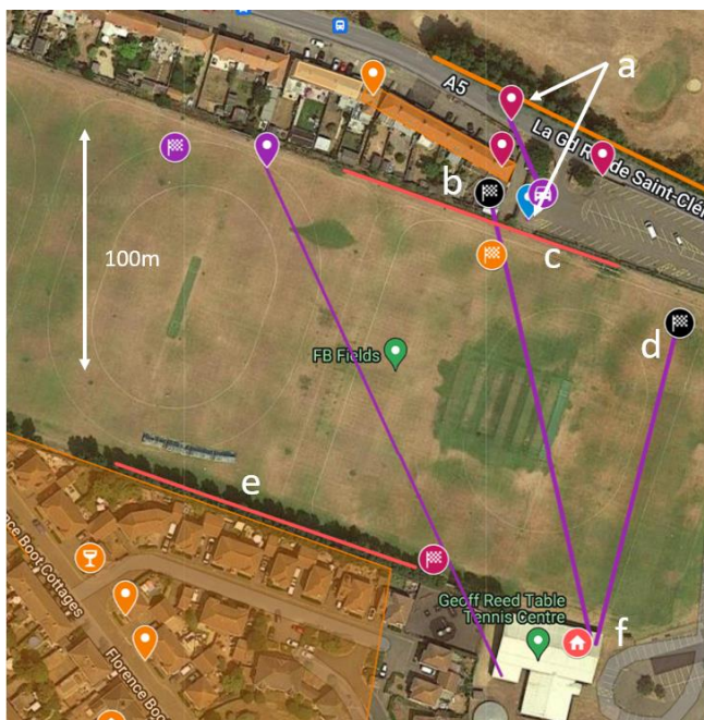
Figure 13: Map of some of the damage found in this area. Most individual damage and debris points are not indicated. Purple lines denote debris travel.
