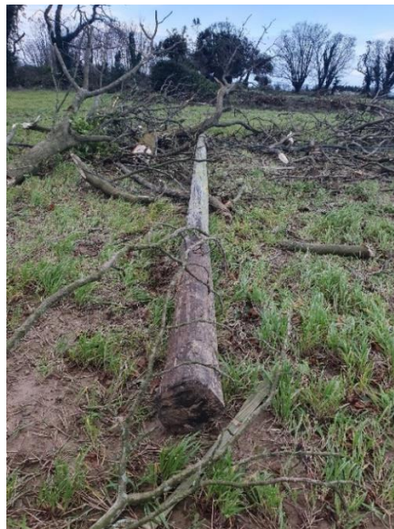
Figure 41: Telegraph pole which had been lifted from the ground, landing around 10m away.
