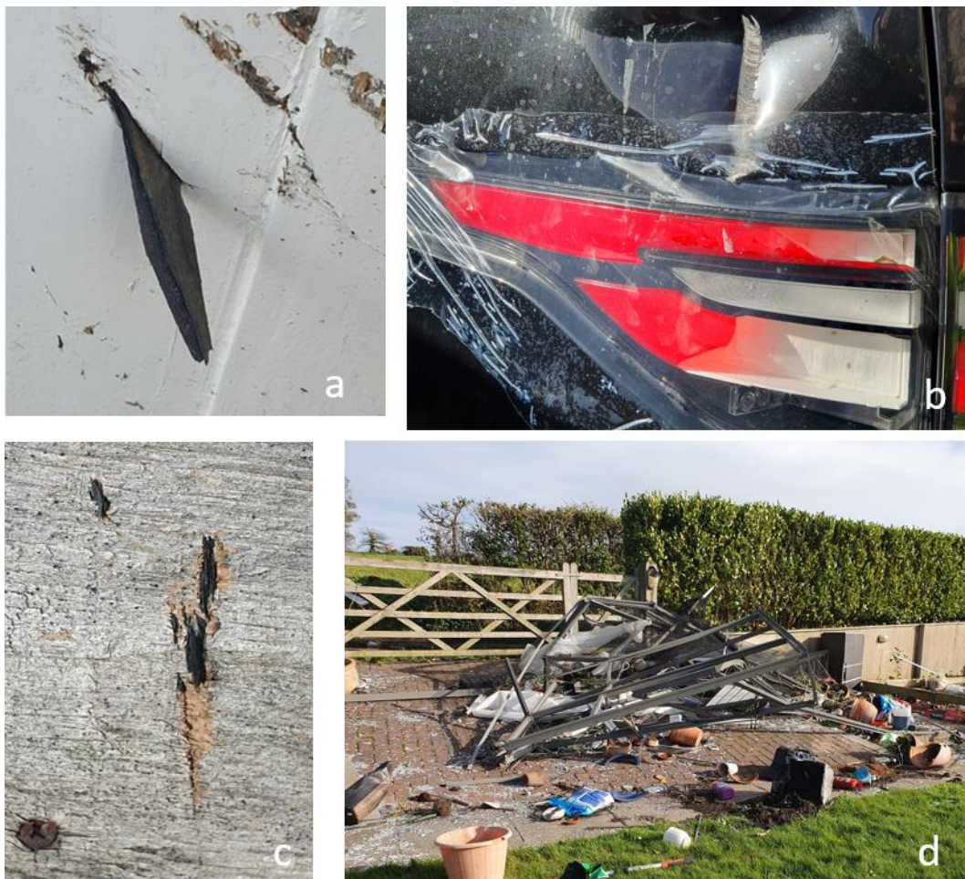
Figure 24: a) and c) show embedded fragments of slate roof tiles in render and wooden sleepers. b) Rear wing of a car showing dents and scrapes from a sharp object. d) A collapsed greenhouse.
