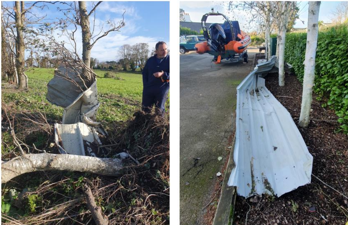
Figure 20: Metal sheeting from the Rue Des Pres Trading estate 1.4km away.
