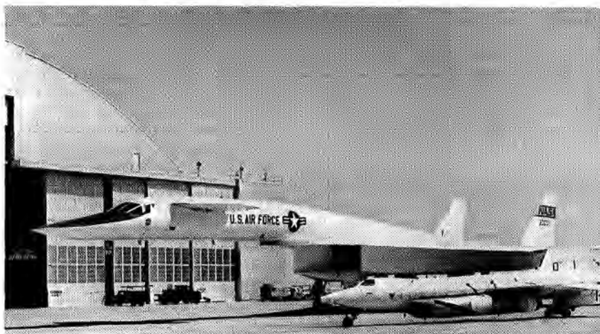
August 21: The X-15 research aircraft stands with the XB-70 research plane outside the hangar at NASA's Flight Research Center. The X-15's new white ablative coating is designed to protect its metal skin from overheating during speeds of more than mach 6.
