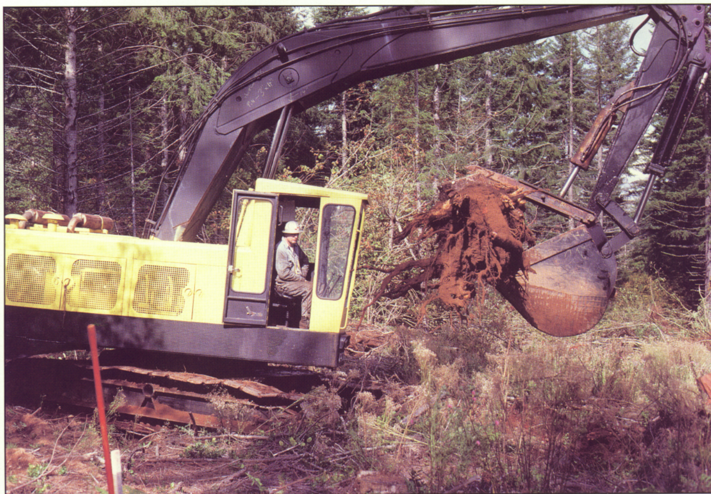
Figure 25—A large excavator with a standard bucket and an optional gripping thumb can be used effectively for stump removal.
