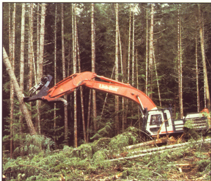
Figure 26—An excavator can be used to push-fall trees.
