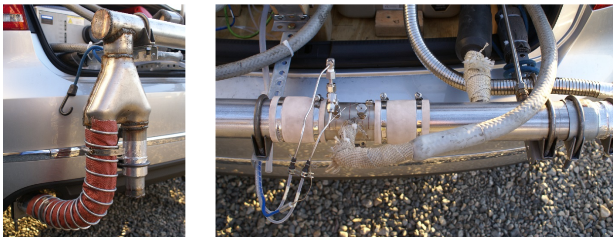
Figure 3.25: Exhaust adapter setup for Vehicle B, left: flexible high temperature exhaust hose connecting single vehicle exhaust tip to exhaust transfer pipe, right: 2" exhaust flow meter (EFM)
