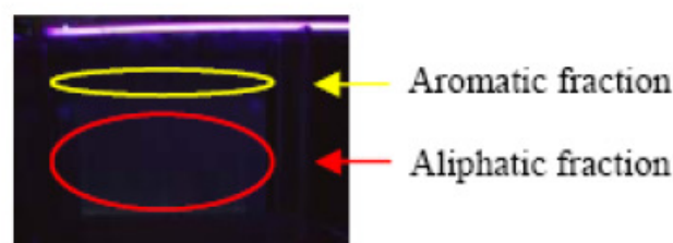
Figure 4: Thin layer chromatography method applied for hydrocarbon analysis.
